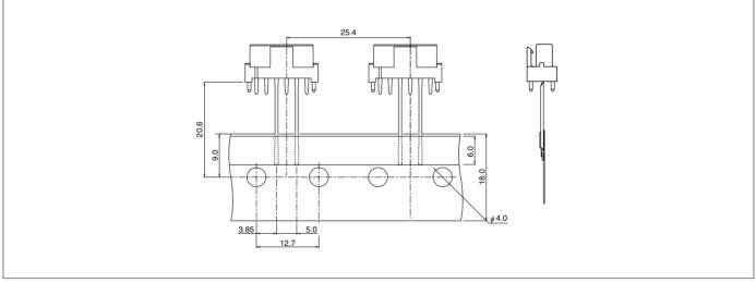
Note: Conforms to JIC C 0806 of "Tape packaging of components with unidirectional leads on continuous tapes".
